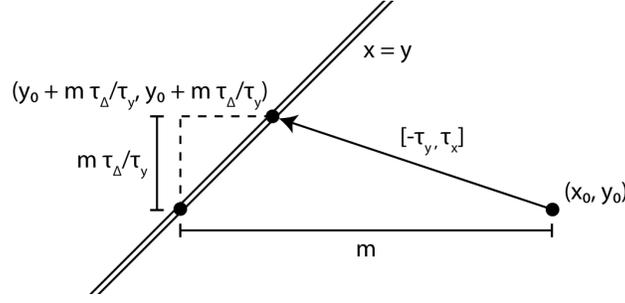
FIGURE 1. Geometric proof of setpoint drift calculation
